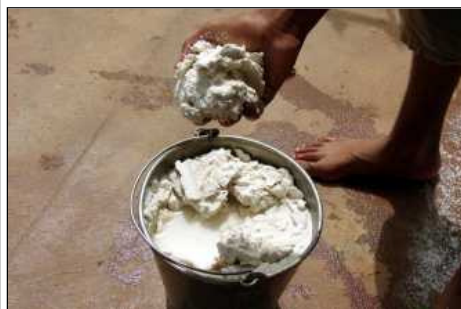
Scales accumulated in corporation water tank. Pic: Shree Padre.
